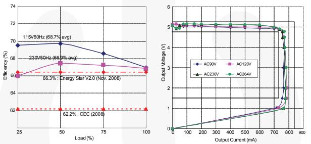
Figure 31. Measured Efficiency and Output Regulation
