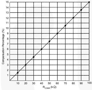
Figure 26. Cable Voltage Drop Compensation
