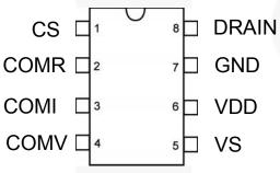
Figure 5. Pin Configuration
