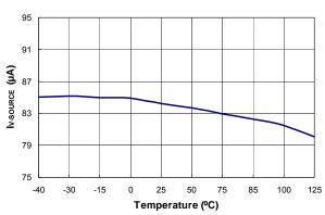
Figure 19. Output Source Current (Iv-source) vs. Temperature
