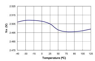
Figure 10. Reference Voltage (V<sub>VR</sub>) vs. Temperature
