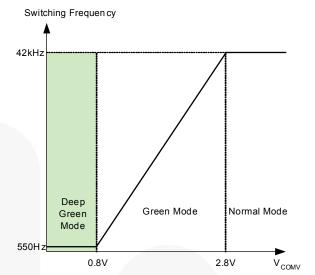
Figure 27. Switching Frequency in Green Mode
