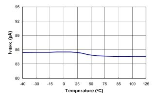
Figure 18. Output Sink Current (I<sub>V-SINK</sub>) vs. Temperature
