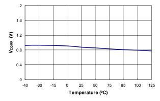
Figure 22. Variation Test Voltage on COMR Pin for Cable Compensation (V<sub>COMR</sub>) vs. Temperature
