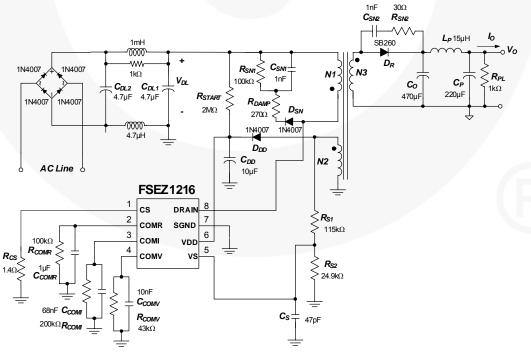
Figure 32. Schematic of Typical Application Circuit
