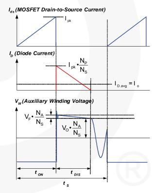
Figure 25. Key Waveforms of DCM Flyback
