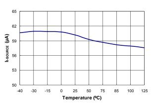
Figure 21. Output Source Current (I<sub>I-SOURCE</sub>) vs. Temperature
