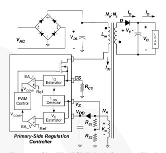
Figure 24. Simplified PSR Flyback Converter Circuit
