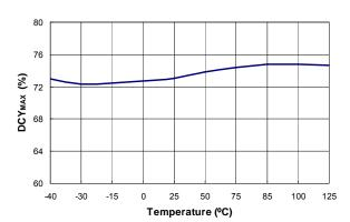
Figure 23. Maximum Duty Cycle (DCY<sub>MAX</sub>) vs. Temperature
