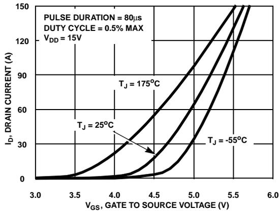
**Figure 7. Transfer Characteristics**
