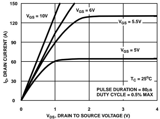
**Figure 8. Saturation Characteristics**
